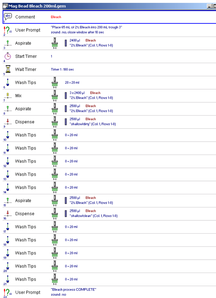
FIG. 4—Script for the 2% bleach routine carried out between each processing step in the overall automation process. This routine takes approximately 15 min to run.
